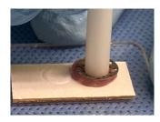
• Finally, the wider end of the assembly tool is used to press the back plate firmly down into the groove, usually with an audible sound. The assembly tool must be perpendicular to the front plate when pressing down.
